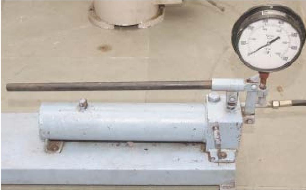
**Figure 2.14: Hydraulic pump for confining pressure**
