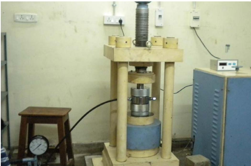
**Figure 2.15: Triaxial testing of cylindrical rock specimen**
