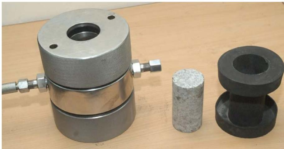
**Figure 2.13: Hoek cell for triaxial testing in rocks**
